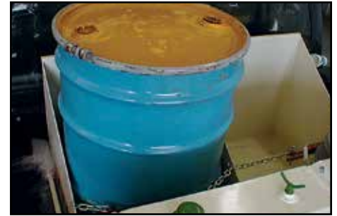
Drum tie-down in lieu of (2) 60 gallon tanks, allows painting directly from drums
