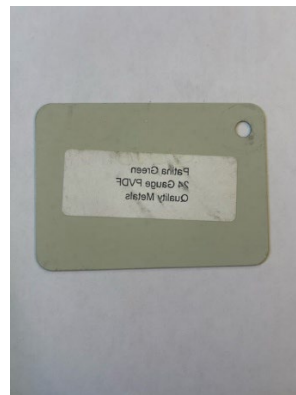
4. – 6. Sample of 24 gauge, double lock, standing seam to be painted in option #1 – Patina Green
