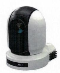
panning, close-ups, and wide shots. The Avior™ HD broadcast-quality robotic cameras are able to tilt and pan through wide angles of motion and can zoom through large ranges.
